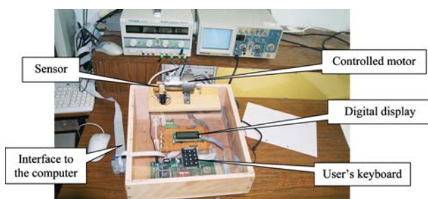
Fig. 1 A typical student project in electronics—a computer-controlled motor
